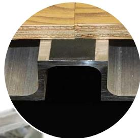
**CONSTRUCTED FOR ENDURANCE:** 3/4", 7-ply marine treated plywood through-bolted and screwed to the hat channels to create the strongest seams in the industry. ("Heavy" hat-channel shown).
