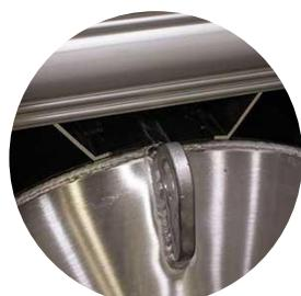
**4-POINT DECK TO HULL FUSION:** Starcraft deck brackets have 4 points of fusion for an extended area of contact with the tube. In addition to providing increased strength and support, this reduces frame twist and racking in rough water and guards against tube fatigue.
