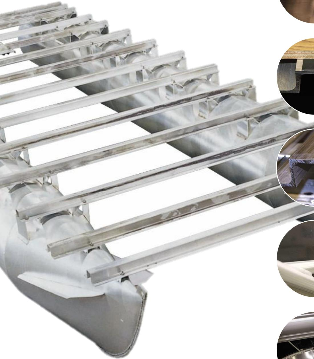
Other manufacturers use C-channel designs which can require more cross members and provide less strength than Starcraft's hat-channel construction. And with imbalanced weight distribution, C-channel cross members are less able to withstand the forces exerted on the pontoon year after year.
