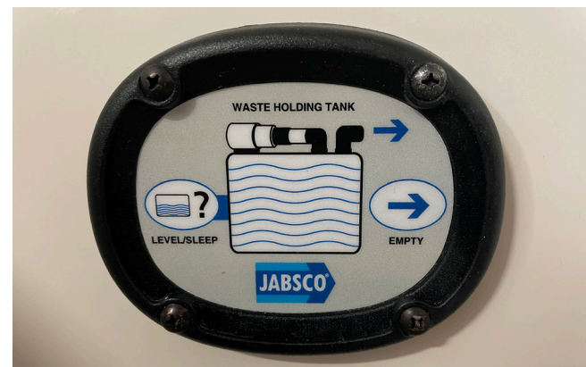
Jabsco Tank Monitor installed with Overboard Discharge Upgrade
