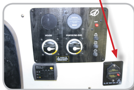
The windlass breaker is located in the head/console compartment.
