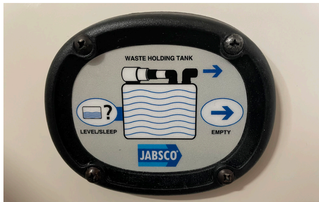
Jabsco Tank Monitor installed with Overboard Discharge
