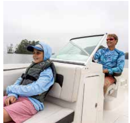
The helm area enjoys the protection of a full windshield, with a center section that swings open for quick access to and from the bow area.
